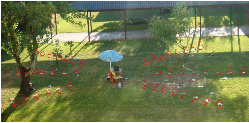
Fig. 4. Nodes distribution according the radial topology, at an outdoor environment.
